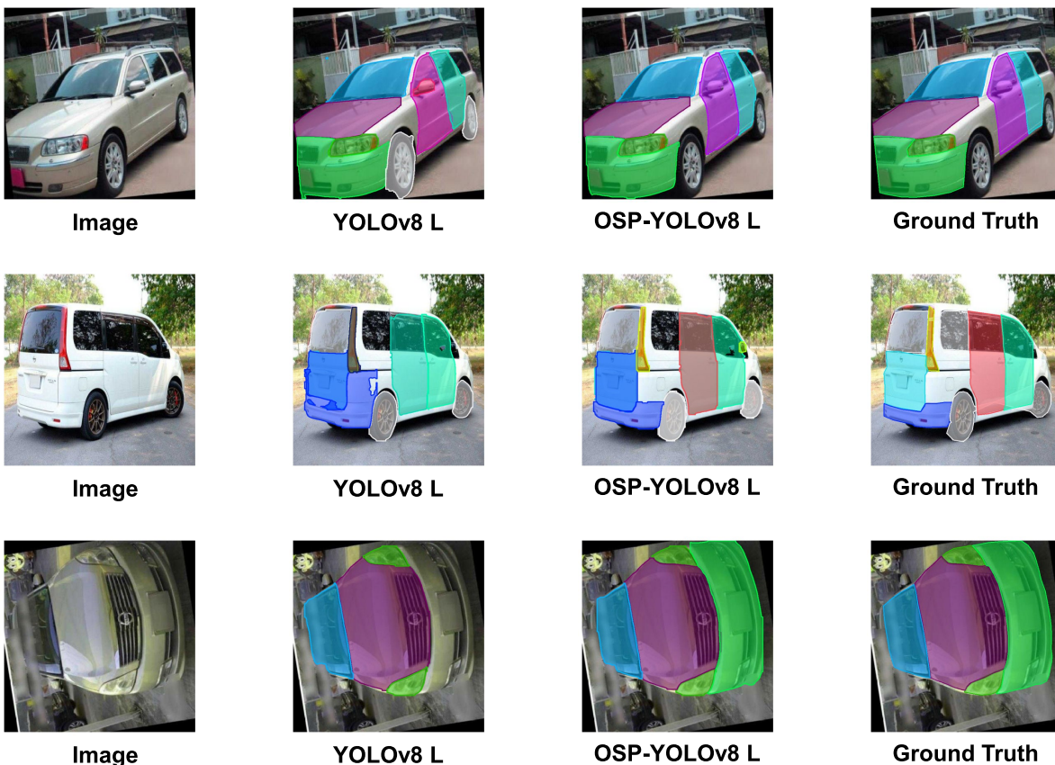
Figure 7. Qualitative comparison on the CarParts dataset. The proposed OSP-YOLOv8 L demonstrates more precise boundary definition and label consistency for individual automotive components compared to the baseline.
